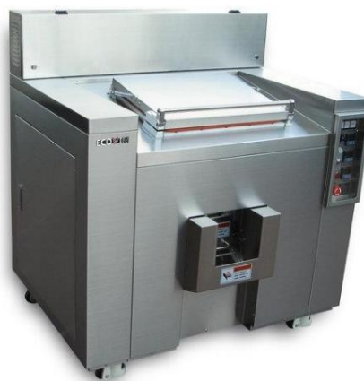
Figure 3 ECOVIM device for processing food waste with a capacity of 100 kg/day (27)
